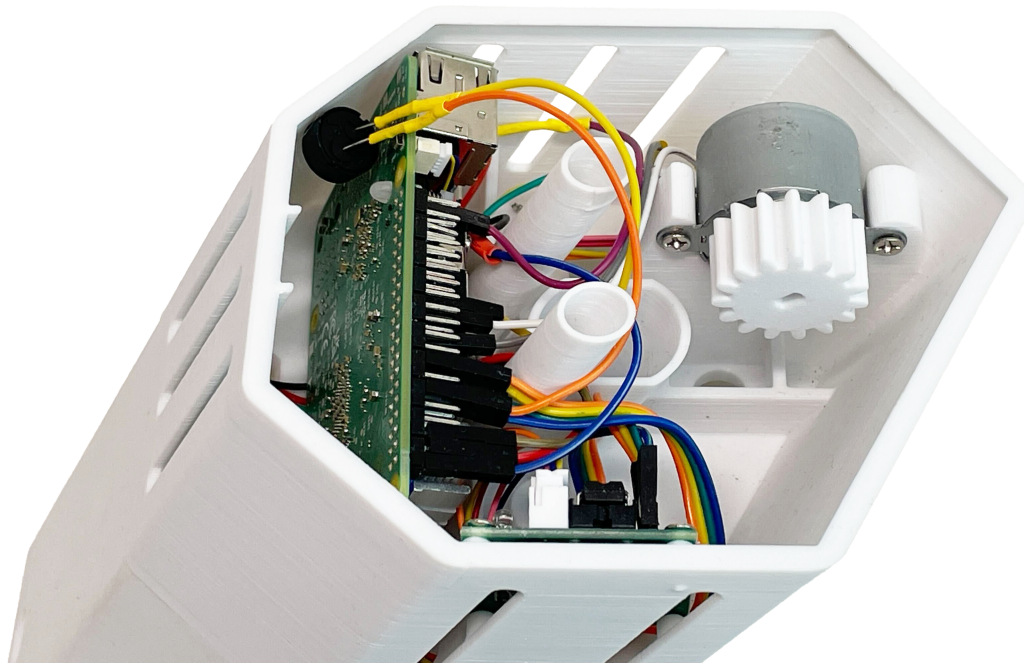
Figure 6: The embedded electronics are arranged diagonally to fit the form design of the WavData Lamp.
